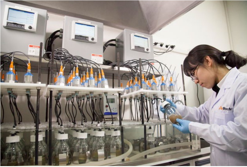
Alltech’s Yea-Sacc® Value Test compares total mixed rations both with and without Yea-Sacc®.
