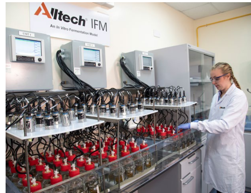
Alltech IFM® simulates rumen fermentation to evaluate the energy and protein availability of feeds.
