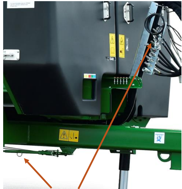
Figure 11: Breakaway safety brake
