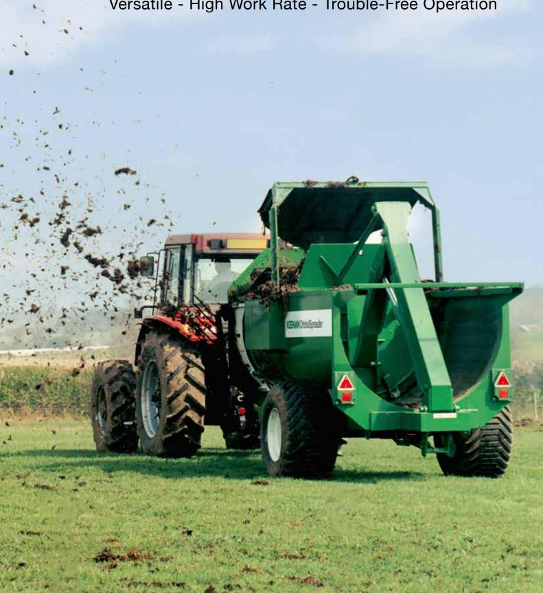
The KEENAN® OrbitalSpreader is a heavy-duty versatile spreader. It is capable of very high work rates with trouble-free operation. Able to handle a wide range of farm and commercial wastes, it delivers a remarkably uniform spread pattern.
