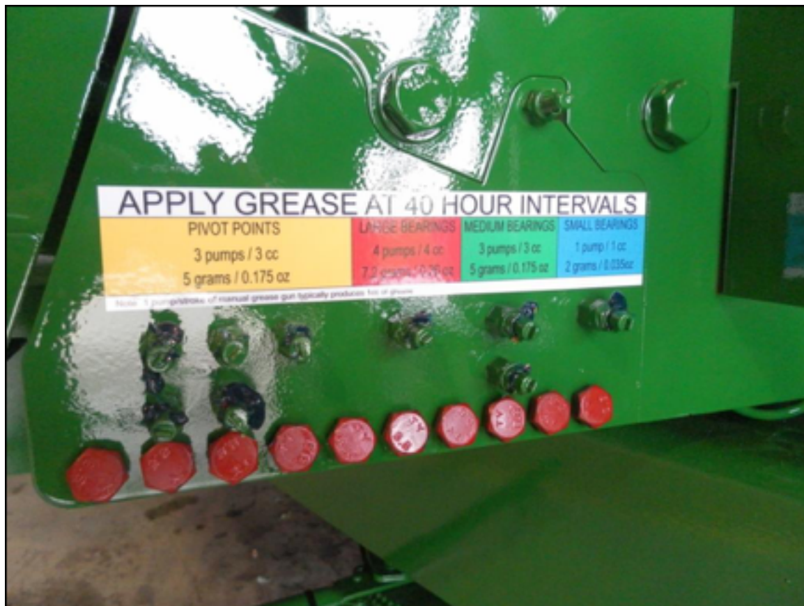
Figure 12: Central greasing manifold
