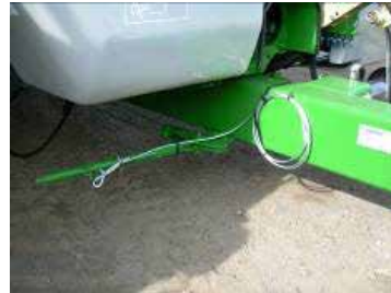
Figure 4: Breakaway Safety Brake
