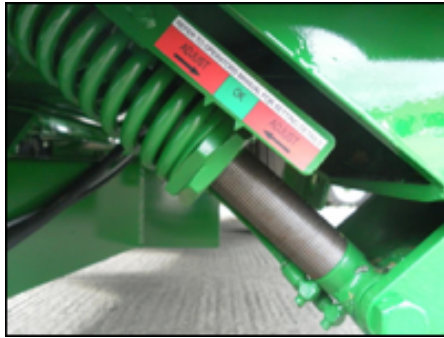
Figure 9.3: Primary chain tensioner adjustment Indicator
