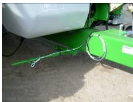
Figure 4: Breakaway Safety Brake
